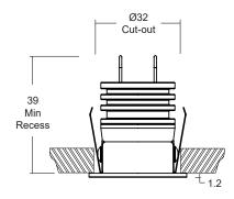
LED and optic position recessed by 10mm for reduced glare.
