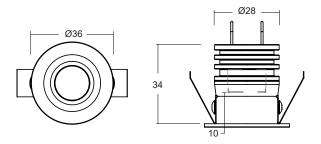
IP54 rated version is supplied with an extra gasket which sits between the bezel and the mounting surface.
